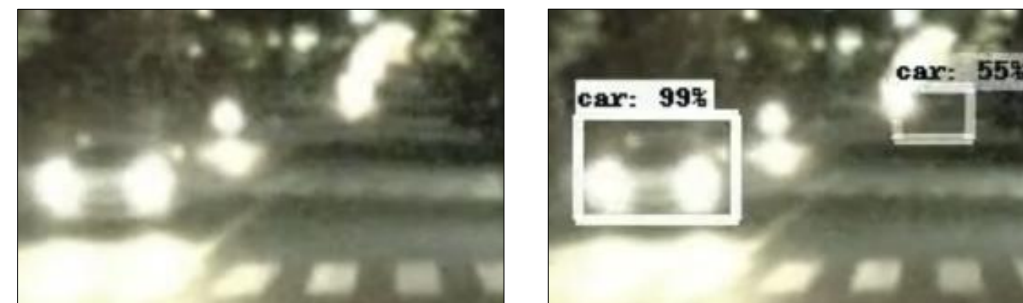
Fig. 2. After wormhole learning (right) we learned to recognize cars only from the headlights.
